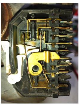
When the two speed motor starts in low speed, the rotational speed is not enough to operate the centrifugal switch, so the start winding is energised continuously. Apart from a nasty noise, this causes excessive heat in the winding and the capacitor. During my learning phase, I destroyed one capacitor this way.
