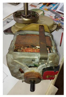
As we are located in Australia, there were a few differences in the wiring from the US machines. Our supply voltage is 240 volts, and the motor is slightly different, but the principle was the same. The motor gearbox assembly is shown left, the motor is part number 3363190.
